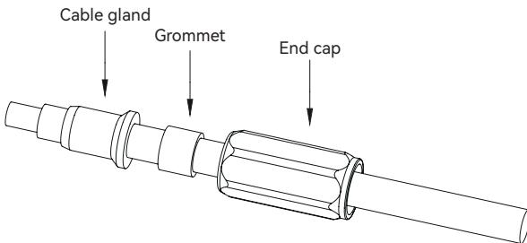
4. Insert the positive and negative cables into the corresponding connectors, and then press the terminal with crimping pliers. After assembling, try to pull back the battery cable to ensure that the terminal is tightly attached in the connector.
