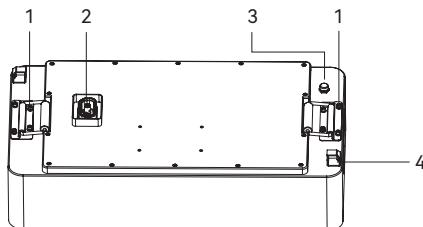
Top View of Battery Module
