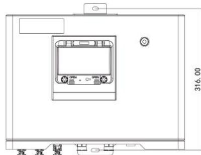
③ Use a Φ8 drill bit for the wall hole 80mm deep, and put expansion tubes into them.
