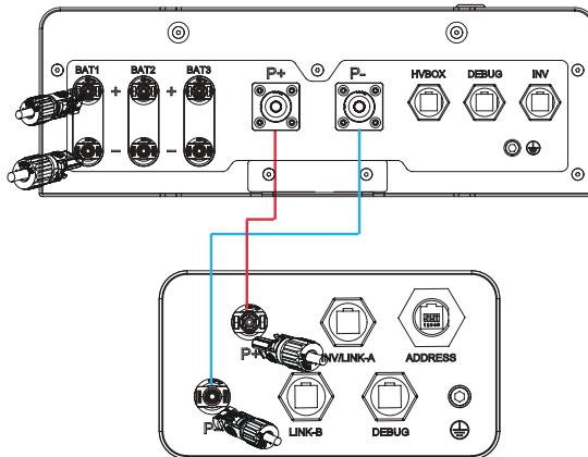
Power cable connection between EBS-P and the inverter procedure is shown as below:
