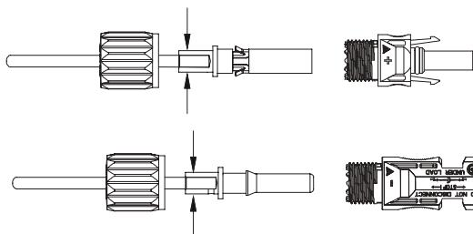
5. Use an open-end wrench to screw the nut to the end to ensure that the terminal is well sealed.
