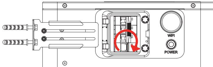
Step2. Hold on “POWER” button for 3 seconds until the indicator becomes green and flashing, which means that the battery enters self-checking.
