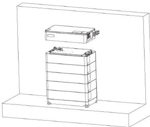
③ Install controller module mounts on both sides of controller module.
