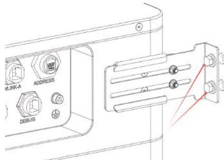
⑩ Turn the adjusting screws to fix the battery onto the wall by using a wrench.
