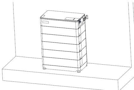
⑧ Tighten all M4\*12 countersunk screws at both side of all battery modules and controller module.
