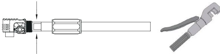
5. After crimping, push the cable gland, grommet and end cap at the plug end into place, and tighten the end cover with the thread of the plug unit.
