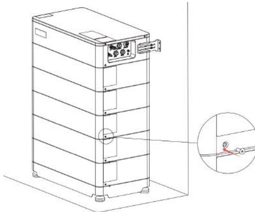
⑨ Insert the expansion screws into the tubes, then fix the mounts onto the wall with expansion screws by using a cross screwdriver.
