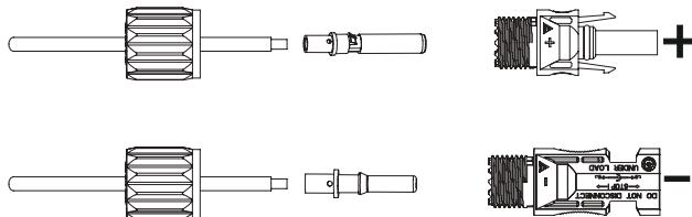
4. Insert the positive and negative cables into the corresponding connectors, and then press the terminal with crimping pliers. After assembling, try to pull back the battery cable to ensure that the terminal is tightly attached in the connector.
