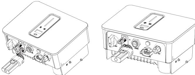
Figure 5-18 Monitoring device installation
