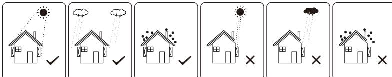
Figure 4-1 Recommended installation location
