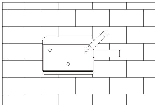
Figure 4-5 Marking hole position using installation bracket
