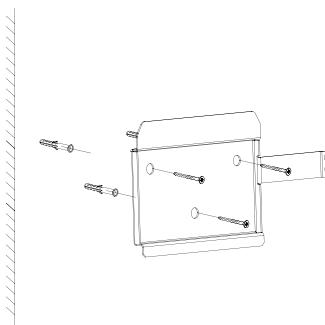
Figure 4-6 Fixing the wall bracket
