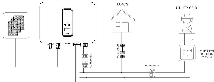
Figure 5-2 Electrical wiring diagram of export limit
