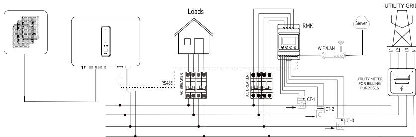
Figure 5-3 Electrical wiring diagram of export limit & 24 hours load consumption monitoring
