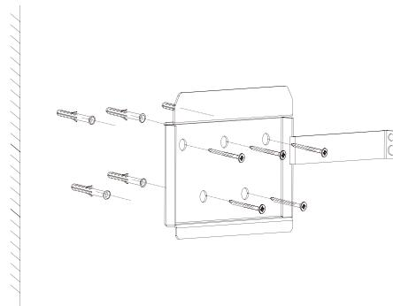
Figure 4-6 Fixing the wall bracket
