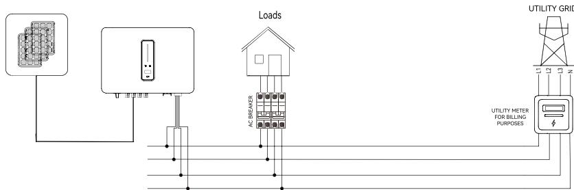
Figure 5-1 Electrical wiring diagram
